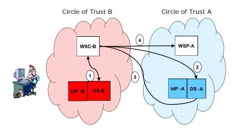
Figure 3: Inter-CoT Access to Id-Based Web Services via Inter-CoT Discovery
